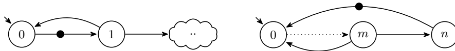
Fig. 2. Worst cases to detect accepting cycle using only one thread. The left automaton is bad for Tarjan since the accepting cycle is always found only after popping state 1. The right one disadvantages Dijkstra since the union of the states represented by dots can be costly.
