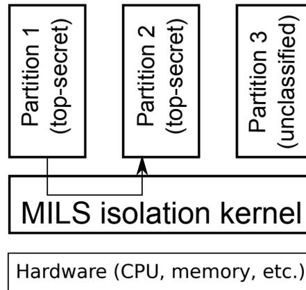
Figure 3. MILS execution platform layers
