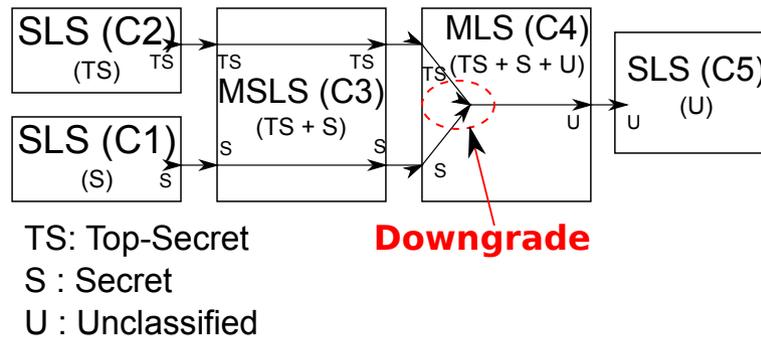
Figure 2. Example of a MILS architecture
