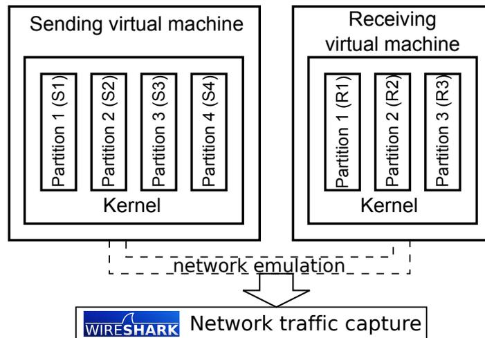
Figure 9. Deployment of our case-study over two virtual machines
