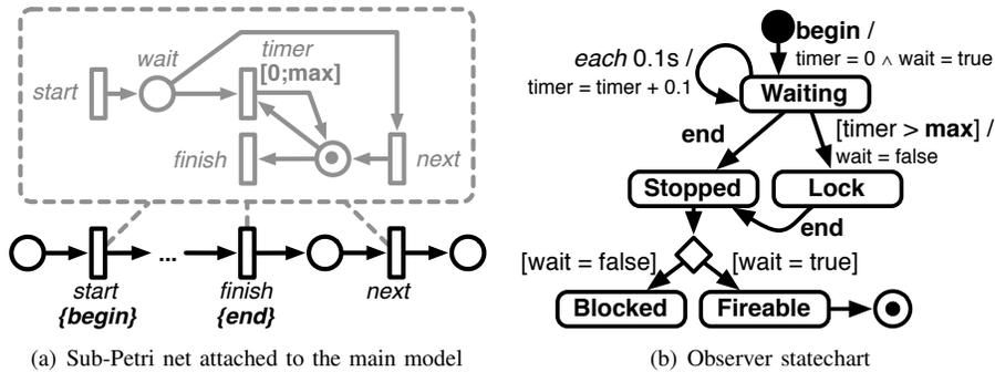
Fig. 5. A temporal-bounds observer that limits the execution time to  $max$  time units
