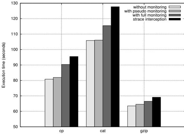
Fig. 7. Monitoring overhead (with and without the firing rule algorithm) for three sequential programs compared to the `strace` performances
