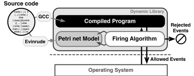
Fig. 4. Architecture of the generated IDS
