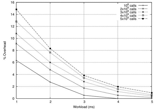
Fig. 9. Runtime overhead for 50 simultaneous clients making  $5 \times 10^6$  requests and considering various server additional workload for the echo-server example
