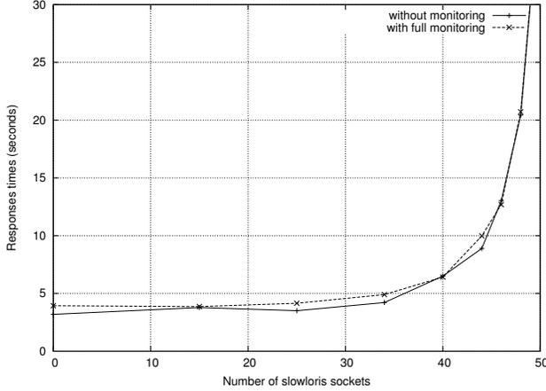
Fig. 10. Response time for 15 simultaneous clients according to the number of connections handled by the client running Slowloris
