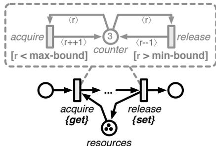
Fig. 6. Sub-Petri net that limits the use of a resource between  $min$  and  $max$
