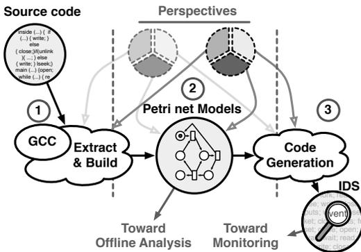
Fig. 1. A three-steps, perspective-driven construction flow
