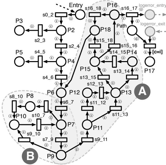
Fig. 2. Structural model built from Listing 2 processing calls and to avoid the “impossible path problem” [7].
