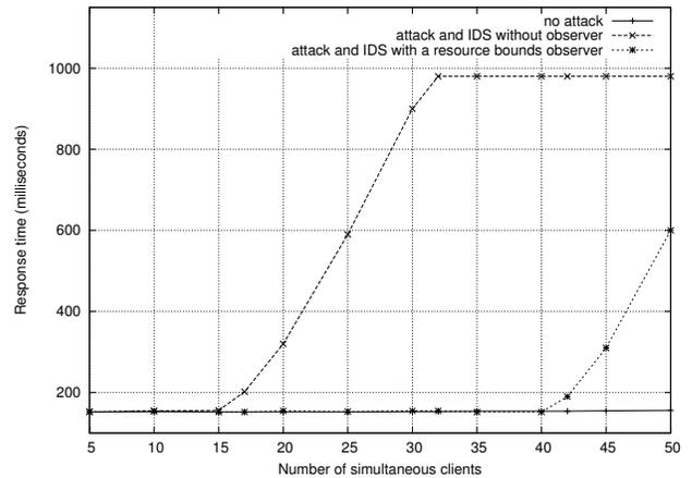
Fig. 12. Response time considering one malicious client handling 35 connections and according to the number of simultaneous clients.
