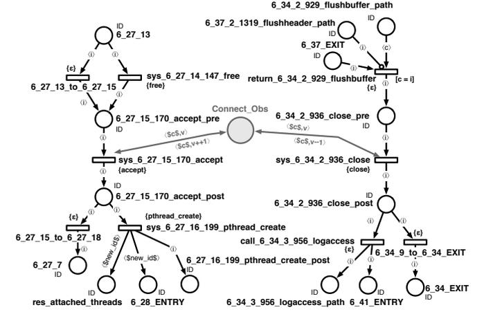
Fig. 11. Resource bounds observer that limit the number of working threads allowed for one client. Only the relevant part of the Petri net describing the reference behavior model is shown here
