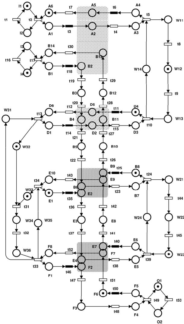
Fig. 1. Petri Net model for 5AGV
