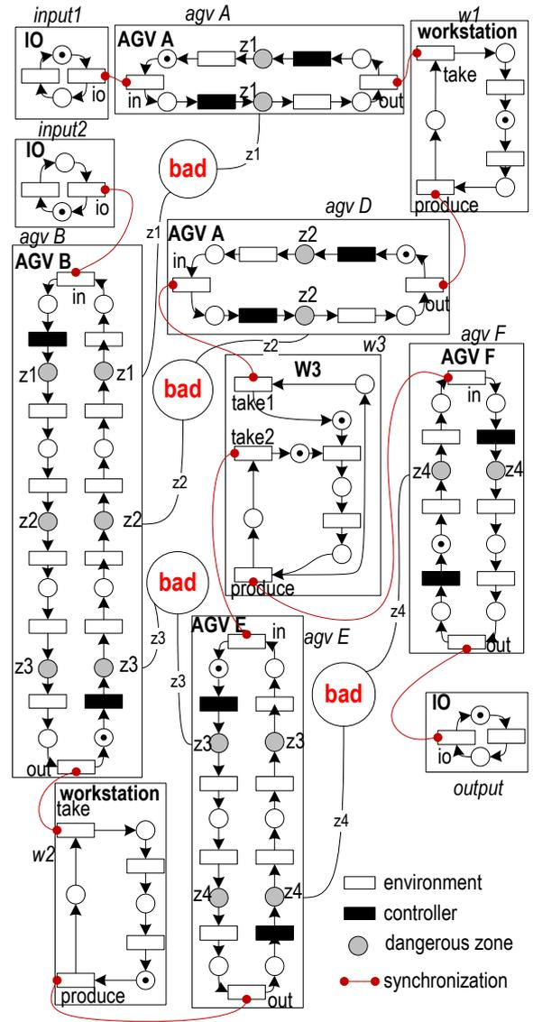
Fig. 2. ITS model for 5AGV
