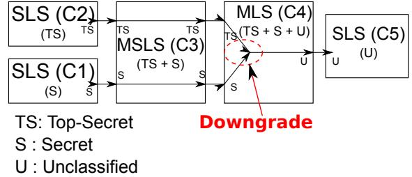
Fig. 2. Example of a MILS architecture
