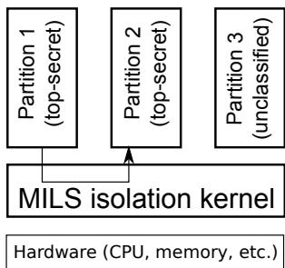
Fig. 3. MILS execution platform layers
