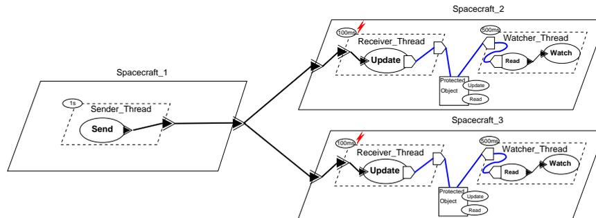
Fig. 4. Software view of the MPC case study
