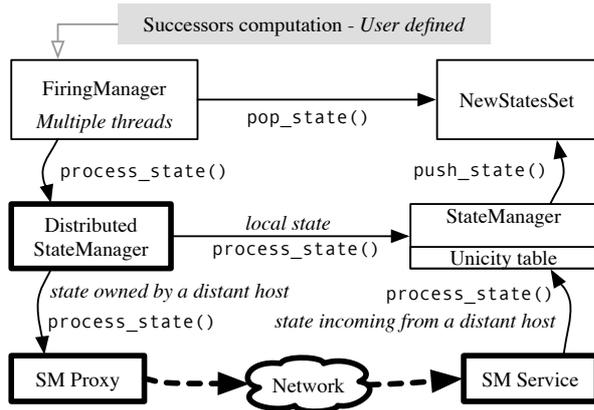
**Figure 2.** libDMC architecture in distributed generation mode
