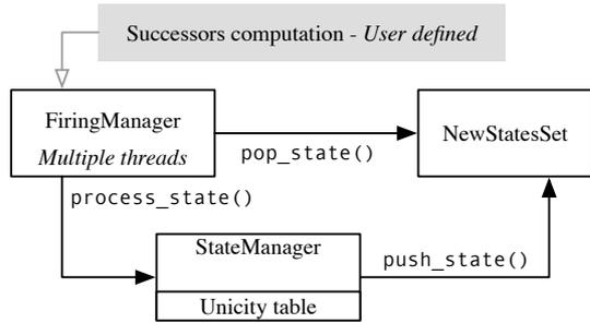
**Figure 1.** libDMC architecture in local generation mode
