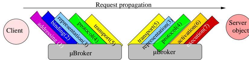
**Fig. 1.** Request propagation in the schizophrenic middleware architecture
