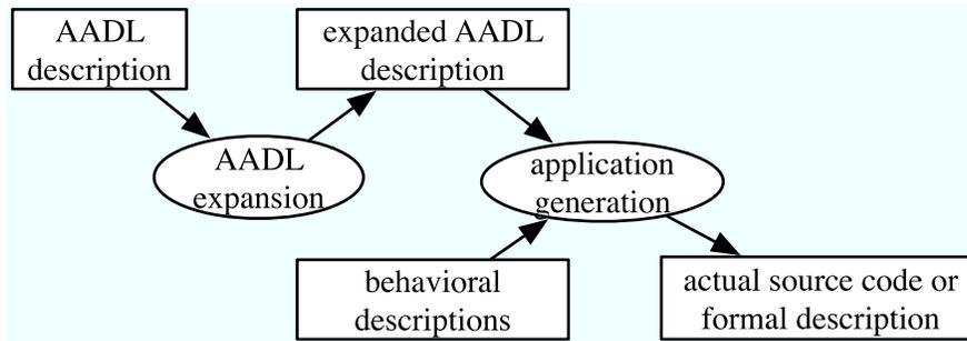
Fig. 5. Application generation based on the AADL
