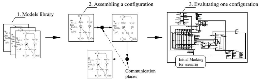
Fig. 4. Steps of the  $\mu$ Broker modeling
