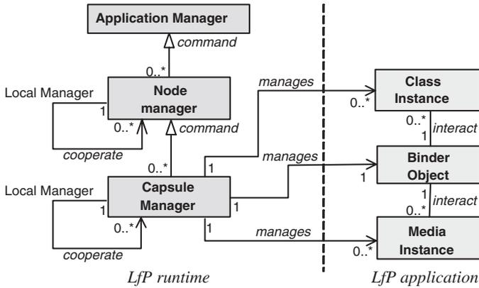
**Fig. 13.** Relationship between the **LfP** runtime and applications.
