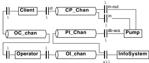
Fig. 3. LfP functional diagram of the gas station.
