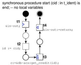
Fig. 7. *LfP*-BD diagram of method *start*.
