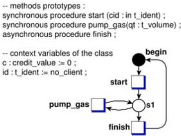
Fig. 6. Behavioral diagram of class *pump*.
