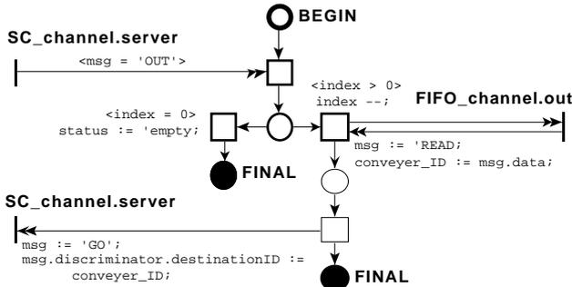
Figure 11 : LfP-FSM of the OUT method.
