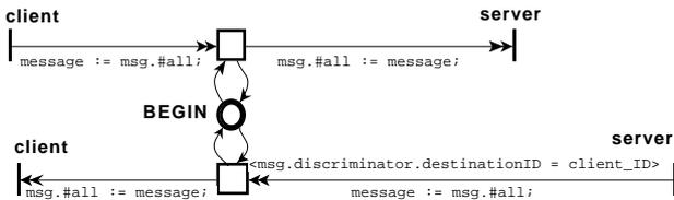
Figure 12 : LfP-FSM of the SC\_channel media.
