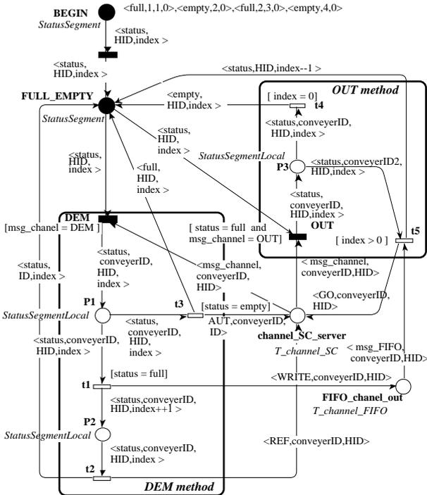
Figure 15 : Petri net of the SC (SegmentControl) class.
