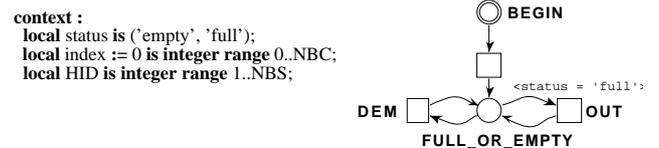
Figure 9 : The main L/P-FSM of the SC class.
