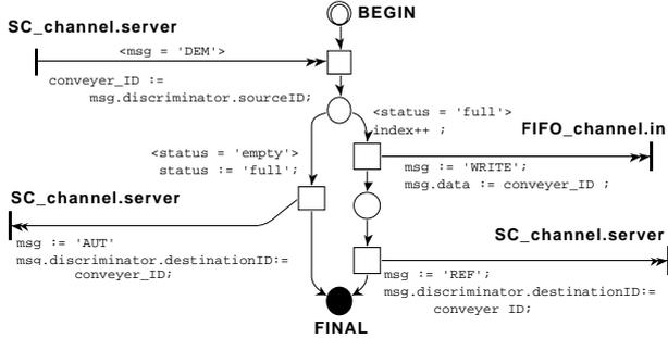
Figure 10 : LfP-FSM of the DEM method.
