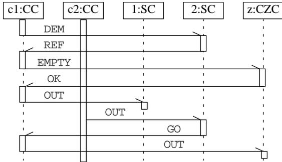
Figure 6 : Sequence diagram of scenario 2.
