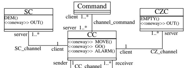
Figure 4 : The UML class diagram of the conveyer system.
